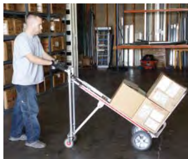
This hand truck fitted with retractable rear wheels converts into a flatbed cart.
