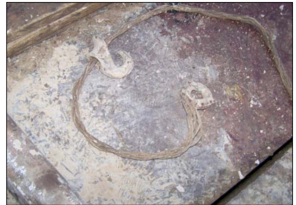
Braided wire rope sling showing signs of wear.
